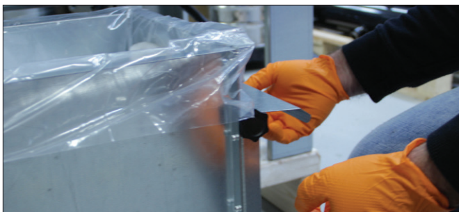
5. Pull down the flap, then it is possible to remove the bag.
