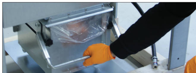
10. Place the bucket back in position and push the handle down while holding the bucket in place. Reconnect the valve to the bucket.
