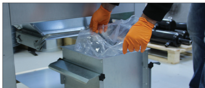
8. Put a new bag in the bucket. Make sure the bag is placed correctly. Avoid breaking the bag when the bucket is placed back in position.
