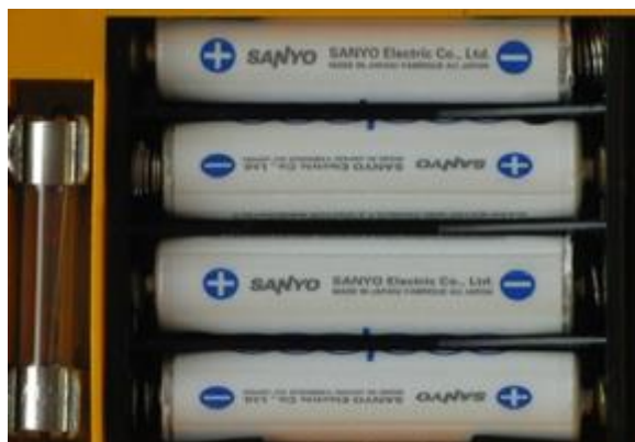
Fig. 4.1 Correct batteries/accumulators polarity and the fuse location
