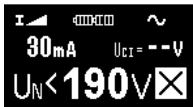
Fig. 3.14 Example of settings for trip-out current measurement
