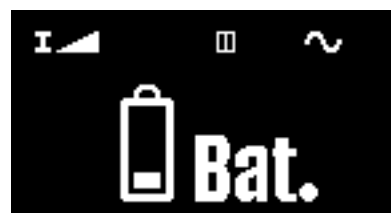
Fig. 3.6b Low battery after the START key was pressed
