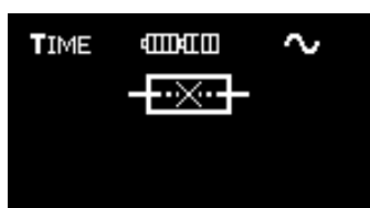
Fig. 3.2 The symbol of blown fuse
