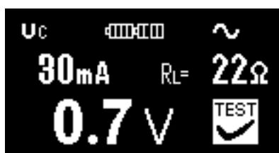
Fig. 3.10 Example of contact voltage measurement result
