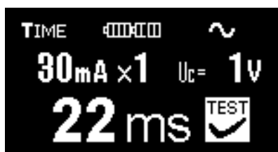
Fig. 3.12a Example of trip-out time measurement result
