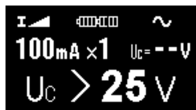
Fig. 3.4b Contact voltage > 25 V
