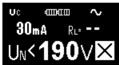
Fig. 3.8 Example of settings for contact voltage measurement
