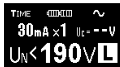
Fig. 3.16b Phase voltage present on the test tip
