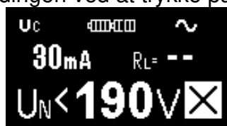
Fig. 3.8 Eksempel for settings for contact voltage measurement
