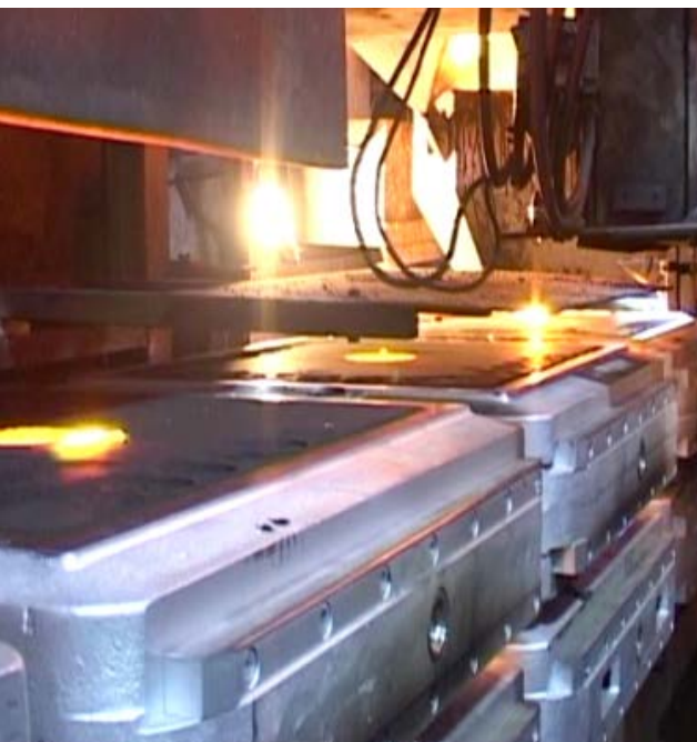
Moulding plant: pouring into the sand moulds
