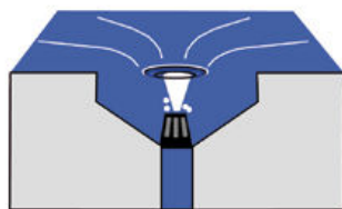
Drain for Aquaperfect siphonic system with air sieve when the calculation rainfall is reached
