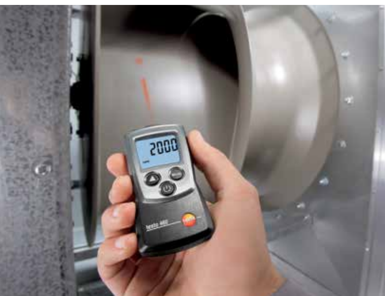
Non-contact measurements on ventilators are possible for example with the handy testo 460. The measurement spot is displayed by an LED marking on the measurement object.
