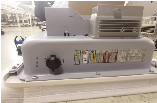
Left side DC switch view
