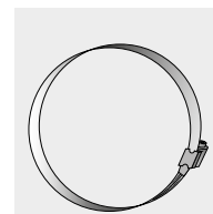
METAL BAND to help cut insulating sheets at the end of large diameter pipes.
